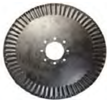
20FL-COMBO 20" Dia Flutes to the edge 8 bolt holes 3-7/16" center hole
