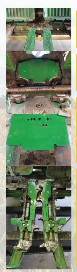
Remove stalk rolls and factory deck plates from the corn head Remove factory chain guides and gathering chains and set aside—if gathering chains have more than about 2-1/2" of droop, replace them. Clean off the decks as shown here, remove all dirt and rust.
